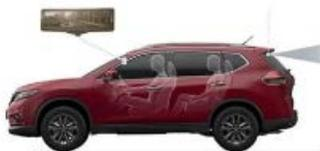
The HD wide rear view image is displayed on the smart mirror, using the images captured by streaming rear view and side view camera modules, as well as the rectification and stitching algorithm. Features of the module include high sensitivity and wide dynamic range, which enables objects to be captured clearly in complicated brightness environment.
